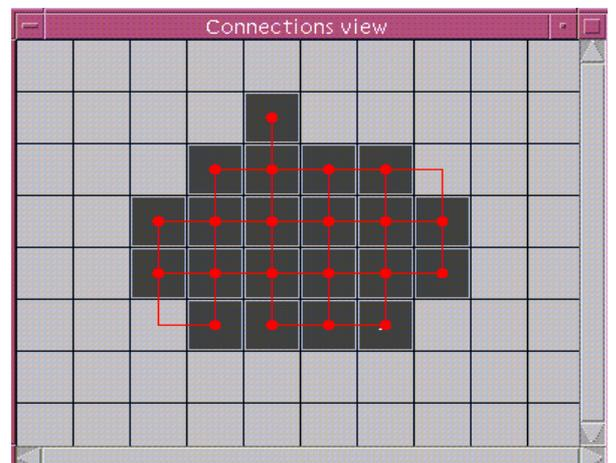
Fig. 6. Component placement with SHORTPATH.
