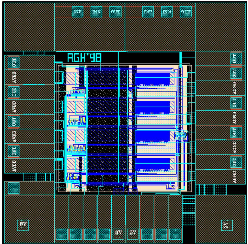
Fig. 9. Test ASIC for active cooling of power ICs.
