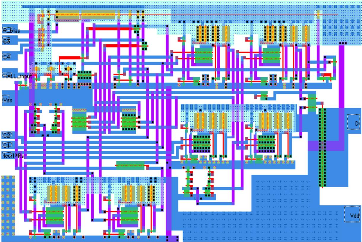
*Fig. 7. Controller for car ignition system.*
